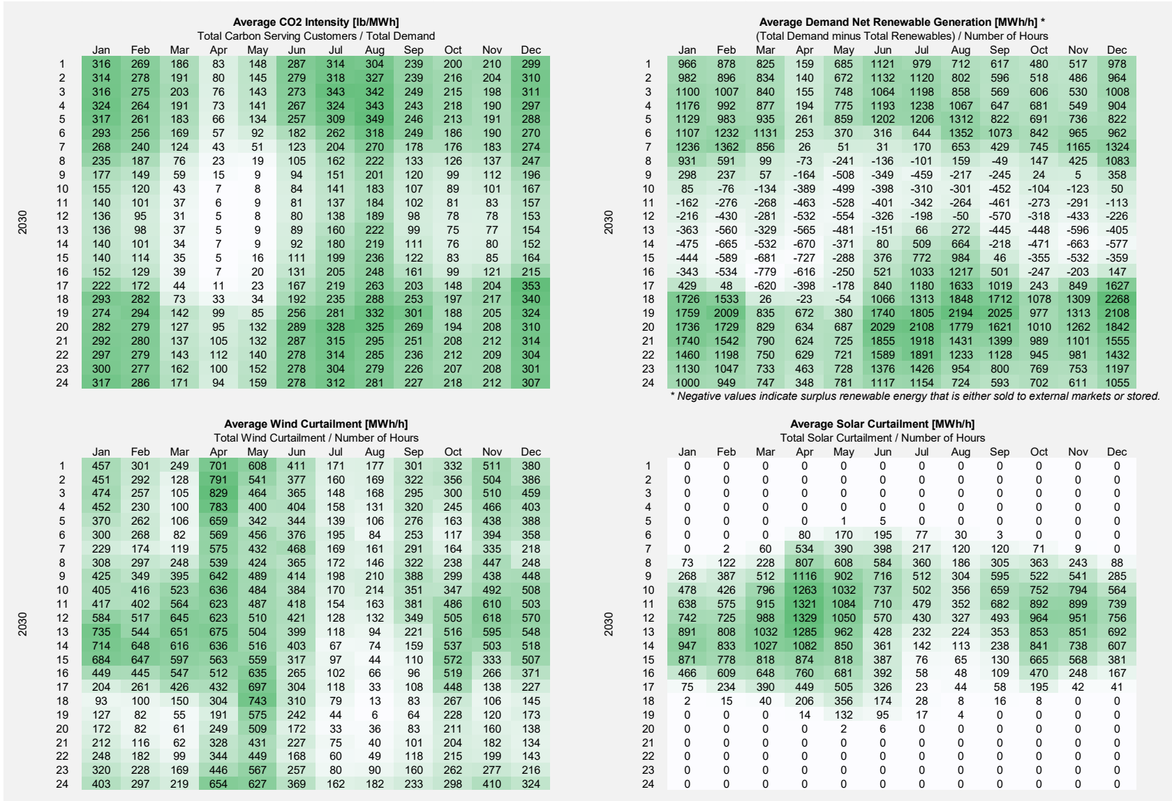
Figure R8 – 2030 Heat Maps of the Modeled Preferred Portfolio: Average CO2 Emissions, Demand Net of Renewables, Curtailment of Wind, and Curtailment of Solar
